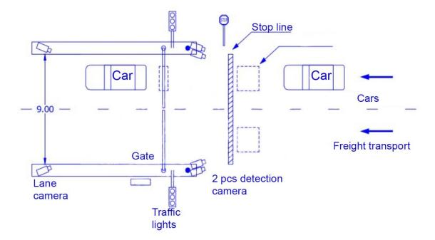
The vehicle drives the identification point over the ground loop, the identification cameras take a picture of the license plate and the access control software identifies the comer.
